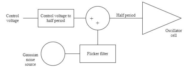
When enable the phase noise, the phase noise is calculated from the variance of the period offset stochastic process from the spectral density at a single frequency. Given the oscillation frequency  $f_0$ , offset frequency f, and single sideband spectral density  $\mathscr{L}(f)$ , the variance of the period offset is:
