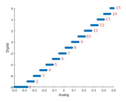
The process for constructing TCR is the same for monotonic or nonmonotonic converters. Once a TCR is created, the function strategically removes the duplicate bins with the smallest number until each digital code corresponds to only one bin. After reducing the TCR, the inldnl function performs analysis on the remaining data.
