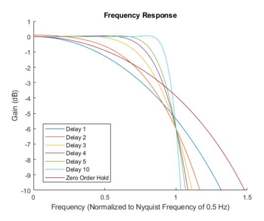
In the time domain, the interpolation does introduce some ringing in the step response of the antialiasing filter, which could affect some digital switching applications. However, the choice of **Number of samples of delay** parameter of 1 and **Output rise/fall time** parameter greater than zero is specifically designed to produce a smooth waveform transition with no ringing.
